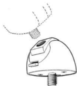
Fig. 8. Northrop-Sierra model B wrist-flexion device.
