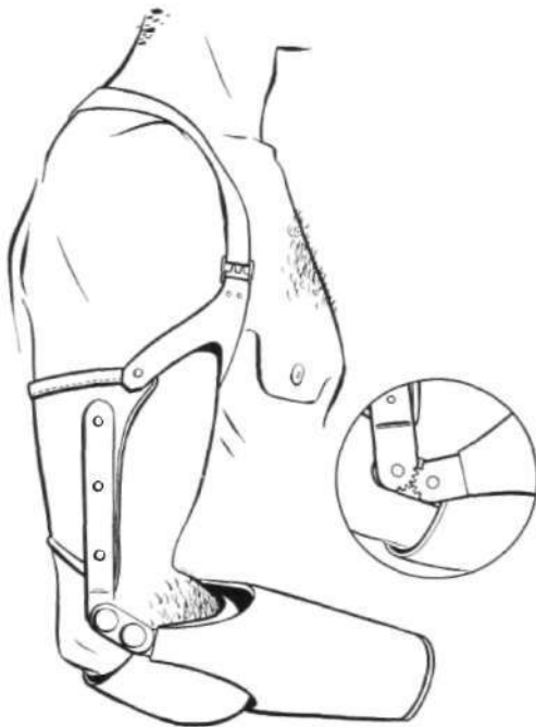
Fig. 11. Hosmer MA-100 step-up hinge.
