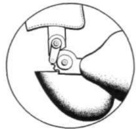
Fig. 12. Robin-Aids stump-actuated elbow lock.
