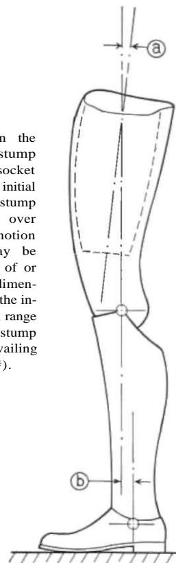
Fig. 7. Alignment in the sagittal plane. The stump should be oriented in the socket with several degrees of initial flexion (*a*) to allow the stump to control knee stability over the widest range of hip motion possible. The ankle may be positioned either in front of or behind the knee. The dimension (*i*) will depend upon the individual amputee, his age, range of motion in the stump, stump musculature, and prevailing terrain. From Haddan(#).
