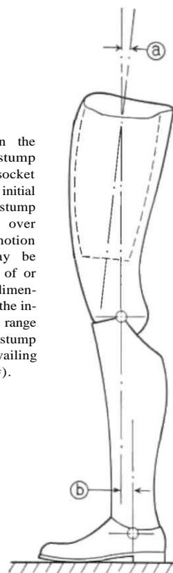
Fig. 7. Alignment in the sagittal plane. The stump should be oriented in the socket with several degrees of initial flexion (a) to allow the stump to control knee stability over the widest range of hip motion possible. The ankle may be positioned either in front of or behind the knee. The dimension (i) will depend upon the individual amputee, his age, range of motion in the stump, stump musculature, and prevailing terrain. From Haddan(#).
