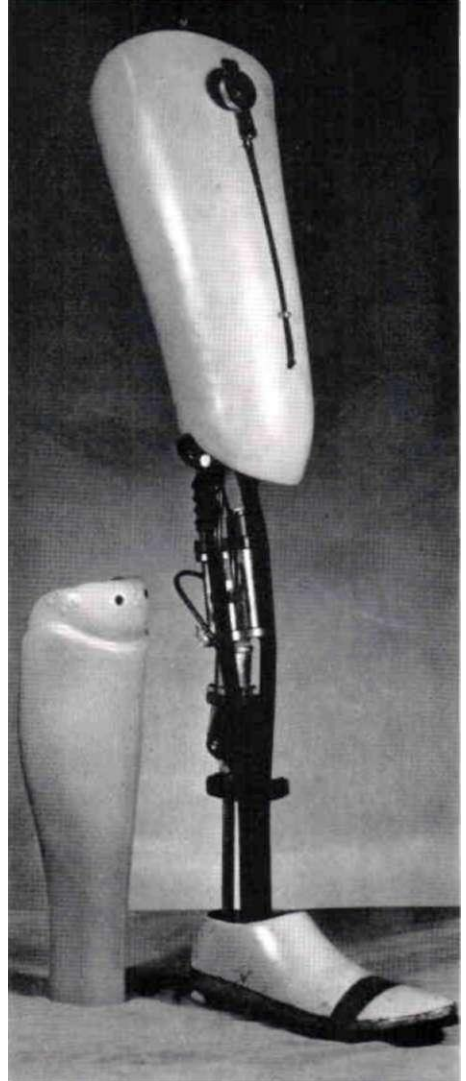
Fig. 9. The Stewart-Vickers hydraulic leg incorporating knee lock, swing-phase control, and coordinated motion between ankle, shank, and thigh. Courtesy Prosthetic Devices Study, New York Unherstity.
