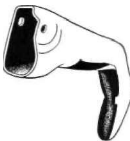
Fig. 10. Artificial finger of monocoque construction with fixed knuckle angles so chosen as to cause grasped objects to be drawn into the hand rather than rejected.
