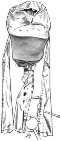
Fig. 16. PVA funnels applied to front and back of lay-up.
