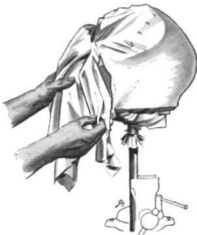
Fig. 13. Final lay-up of dacron fabric.
