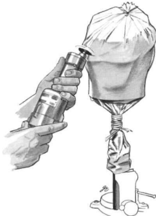
Fig. 21. Cutting the socket free of the mold.
