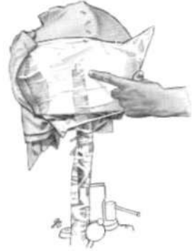
Fig. 14. Application of PVA funnel and film separator under overlap of waistband.
