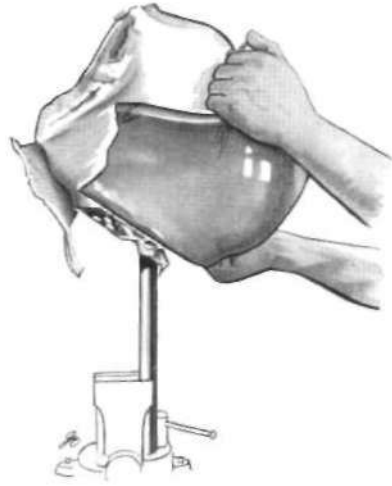
Fig. 22. Removing the socket from the mold.
