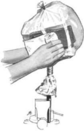
Fig. 20. Sponge-rubber pads applied to undercut areas to guarantee adherence to mold.
