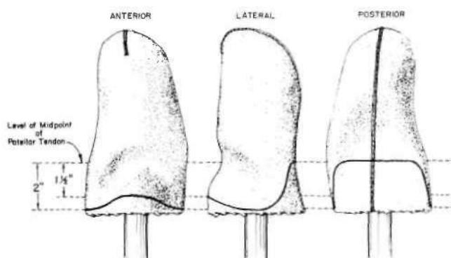
Fig. 11. Proximal trim line of the leather liner,
