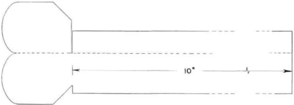
Fig. 69. Pattern for side-joint covers, half actual size.
