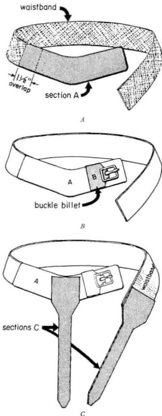
Fig. 73. Details of assembly of the pelvic belt.
