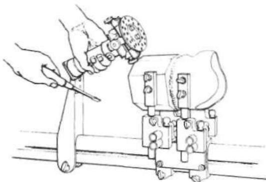
Fig. 44. Removal of the adjustable shank.
