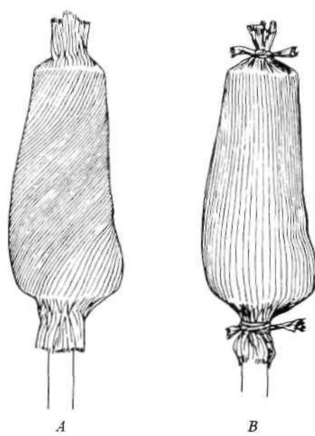
Fig. 54. Layup for lamination of socket-shank combination. *A*, First of two layers of nylon stockinet twisted over layer of Fiberglas cloth; *B*, second layer of nylon stockinet applied and tied off at both ends.
