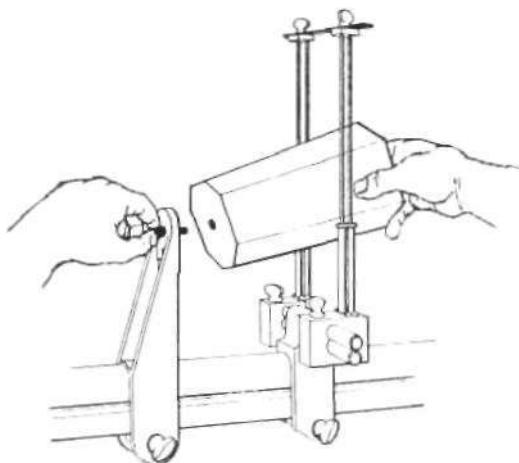
Fig. 47. Attachment of shank block to ankle bracket.
