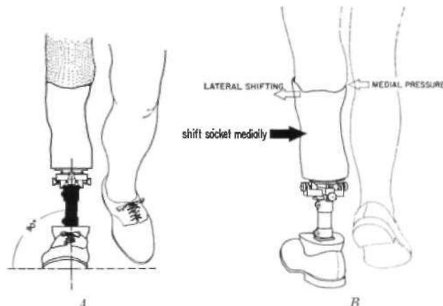
Fig. 36. Check of foot and socket in mediolateral plane during walking. A. Proper alignment in front view; B, correction for undue pressure at medial brim of socket, rear view. Compare with Figure 34A.
