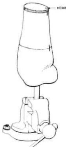
Fig. 53. Application of disc of Kemblo to end of shank prior to layup and lamination.
