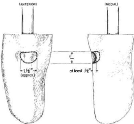
Fig. 5. Initial step in modification of the positive mode]—undercutting to enhance support on patellar ligament.
