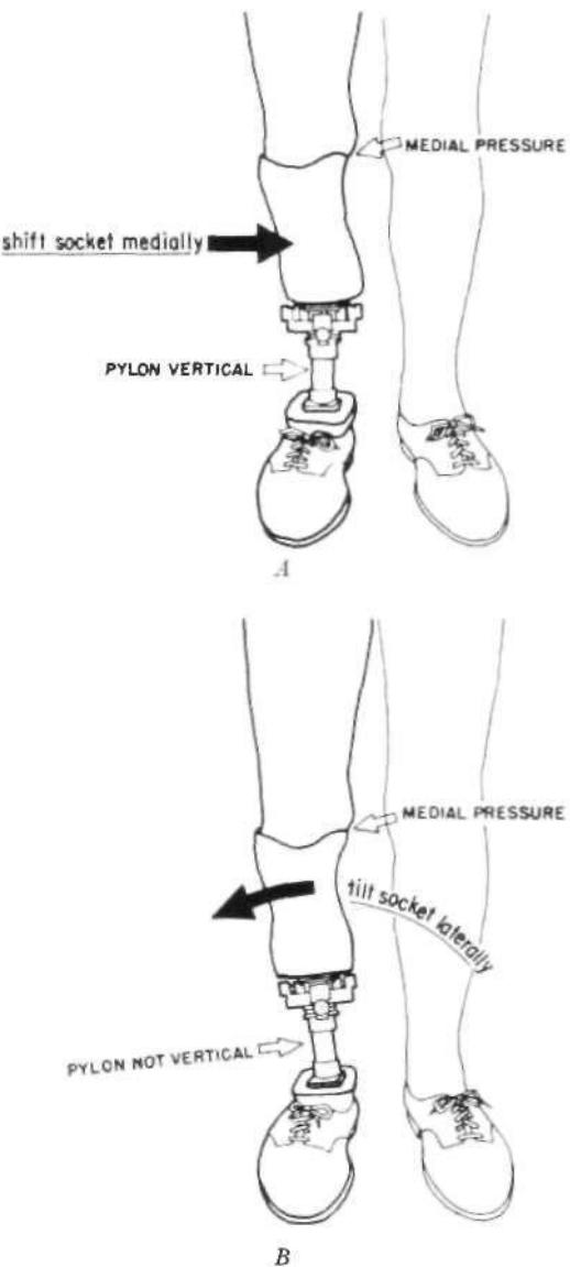
Fig. 34. Two faults in mediolateral alignment sometimes found during initial trials of prosthesis on amputee. A, Pylon vertical (foot flat on floor) but socket too far lateral; B, same situation but with pylon tilted laterally so that foot rests on outside edge of sole only.
