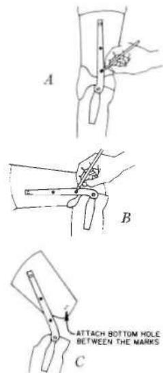
Fig. 64. Tentative attachment of upper sidebar straps to corset.
