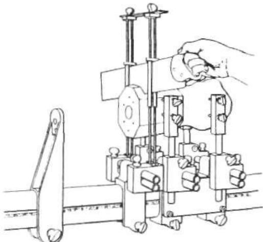
Fig. 46. Making saw cut on bottom of socket block. Remove not more than 1/4 in. at thinnest point about periphery.
