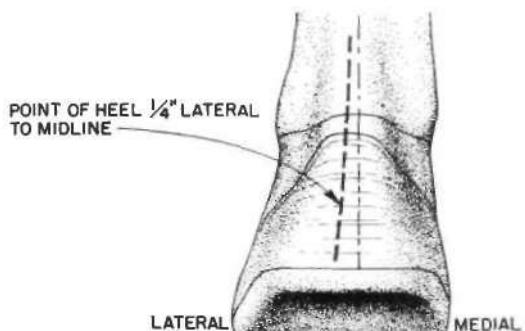
Fig. 25. Shaping of the heel of the SACH foot to accommodate toe-out in the finished prosthesis.
