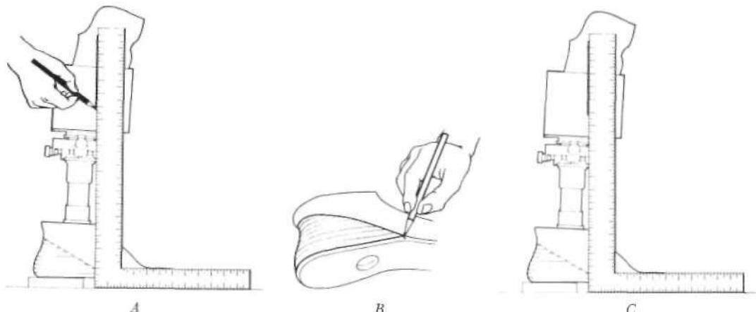
Fig. 1. Method of changing heel cushion in SACH foot whenever cushion is found to be too soft or too stiff. A, Recording existing alignment (to be preserved); B, marking about sole of heel to establish anterior point of heel wedge (also to be maintained); C, checking alignment after new cushion has been inserted.
