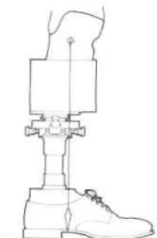
Fig. 39. Ultimate anteroposterior position of socket with respect to shoe. A plumb line dropped from the anteroposterior centerline of the socket at the level of the midpatellar tendon should pass just ahead of the breast of the heel of the shoe.
