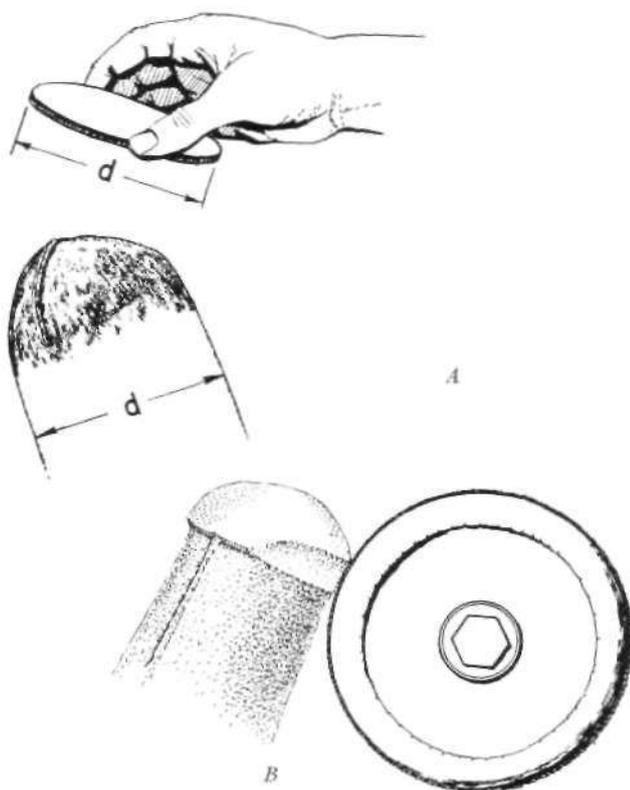
Fig. 12. Construction of the socket end pad.
