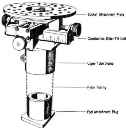
Fig. 18. The University of California below-knee adjustable shank.
