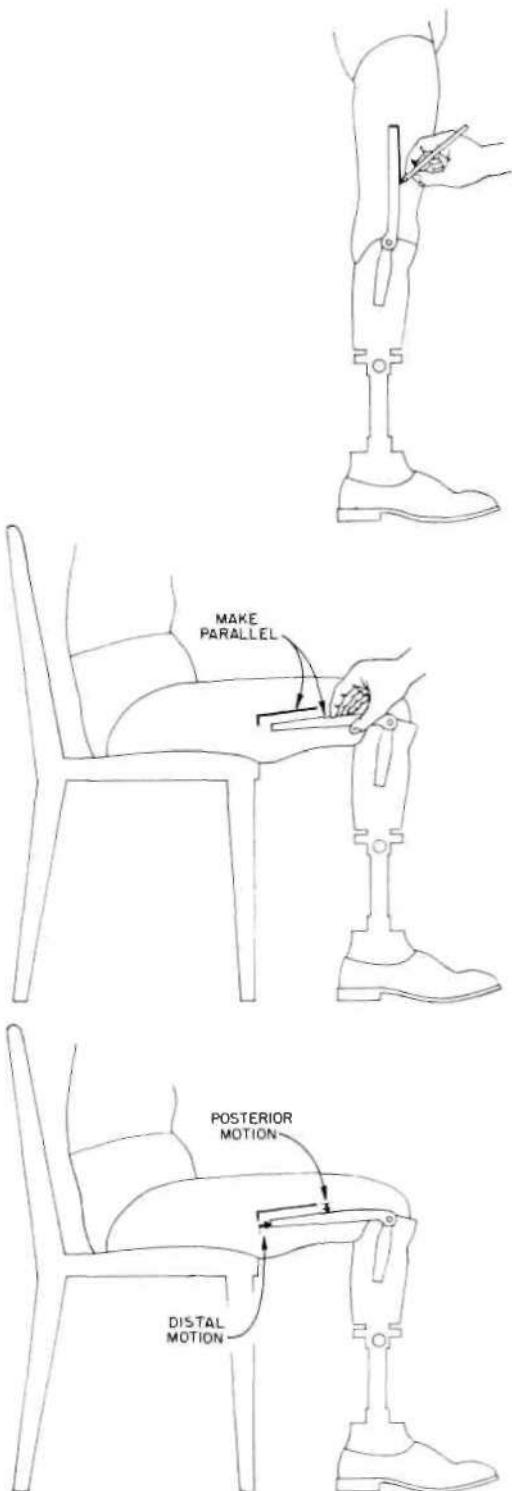
a close fit here helps to suspend the prosthesis. At this point the corset is cut to shape and is temporarily attached to the upper sidebars of the joints with binding screws.
