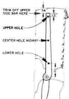
Fig. 63. Preparation of upper sidebar straps for later attachment to leather thigh corset.
