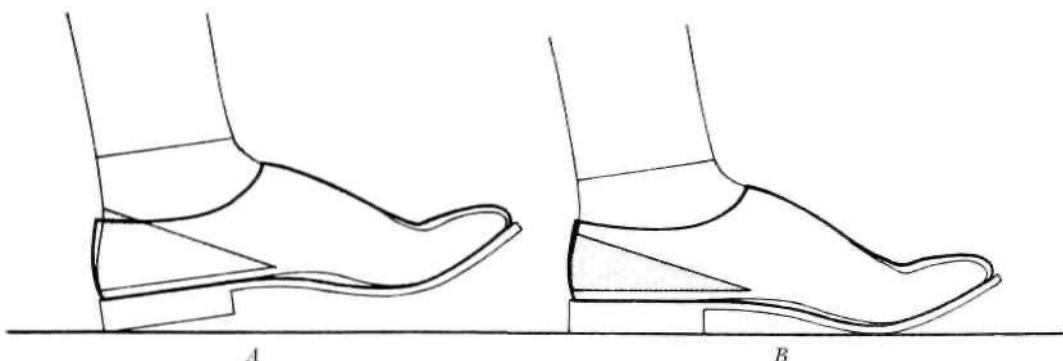
Fig. 23. The SACH foot, in transparent shoe, schematic. A, Heel contact; B, plantar flexion immediately after heel contact, heel wedge compressed. Rocker shape of keel at the ball of the foot gives support during roll-over and furnishes needed assistance at toe-off. Flexible toe piece permits normal toe-break in the shoe.
