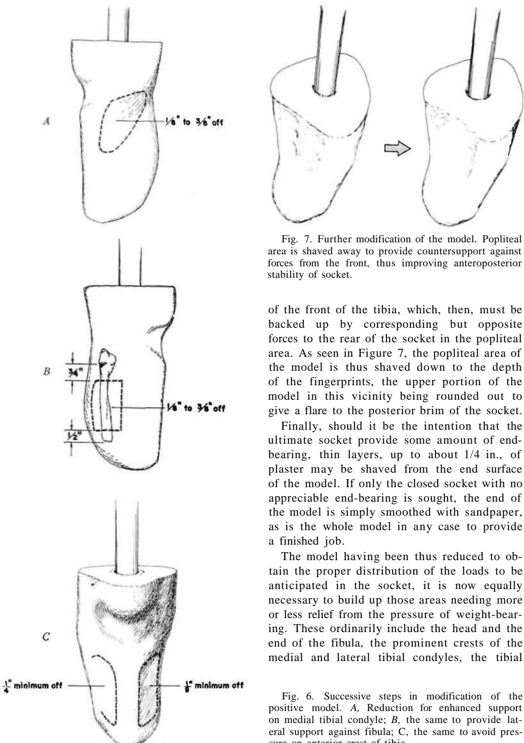
Fig. 7. Further modification of the model. Popliteal area is shaved away to provide countersupport against forces from the front, thus improving anteroposterior stability of socket.
