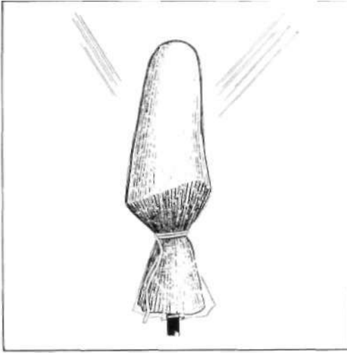
Fig. 9. The stockinet layup on the model. A PVA sheet is pulled down and tied at the base rod.
