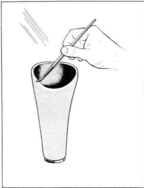
Fig. 7. Bonding the socket and forearm.
