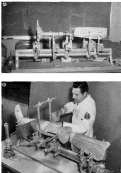
Fig. 3. Alignment duplication jig. A, Adjustable leg mounted in jig. B, Adjustable leg has been removed and wooden set-up substituted. Prosthetist is sawing shank to proper length.
