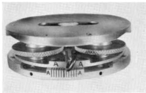
Fig. 4. The adjustable coupling assembled.
