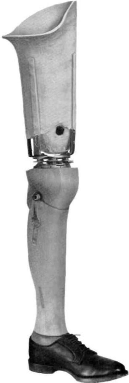
Fig. 16. The adjustable coupling used with a plaster of-Paris above-knee temporary socket and an unfinished knee shank. The three straps are each 1/8 in by 3/4 in. low-carbon steel. From (9).
