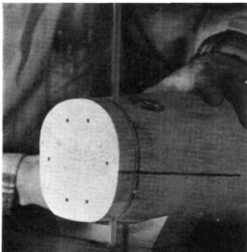
Fig. 11. Using the band-saw to cut the socket immediately below the horizontal-circumferential reference line.
