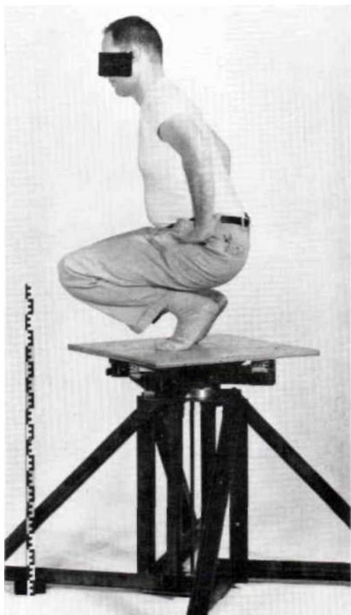
Fig. 20. Mass moment of inertia determination (squatting position).
