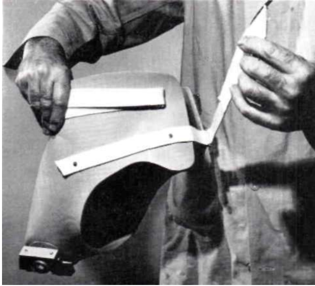
Fig. 25. Arrangement of closure straps using Velcro.
