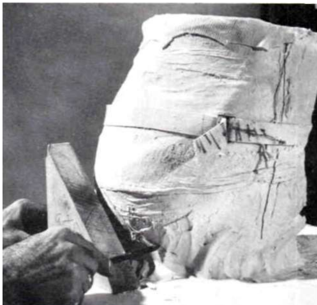
Fig. 14. Scribing 45-deg. line on cast.
