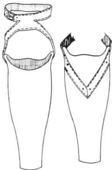
Fig. 1. Anterior and posterior views of typical cuff-suspension system for PTB prosthesis.
