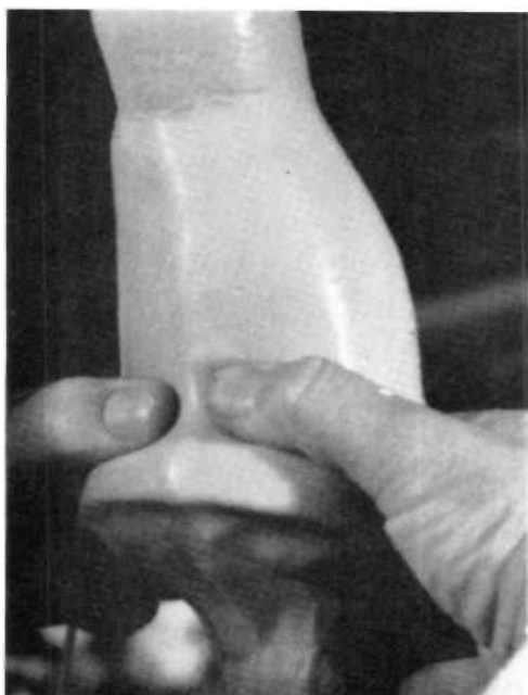
Fig. 42. Working resin into undercut areas.
