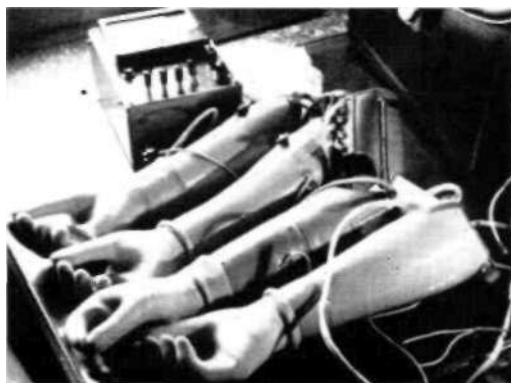
Four standard electrically powered Russian arms that are actuated by electromyographic controls. Courtesy of James B. Reswick.
