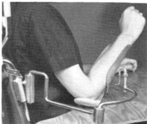
Fig. 8. Segmented-arm feeder of October 1952.
