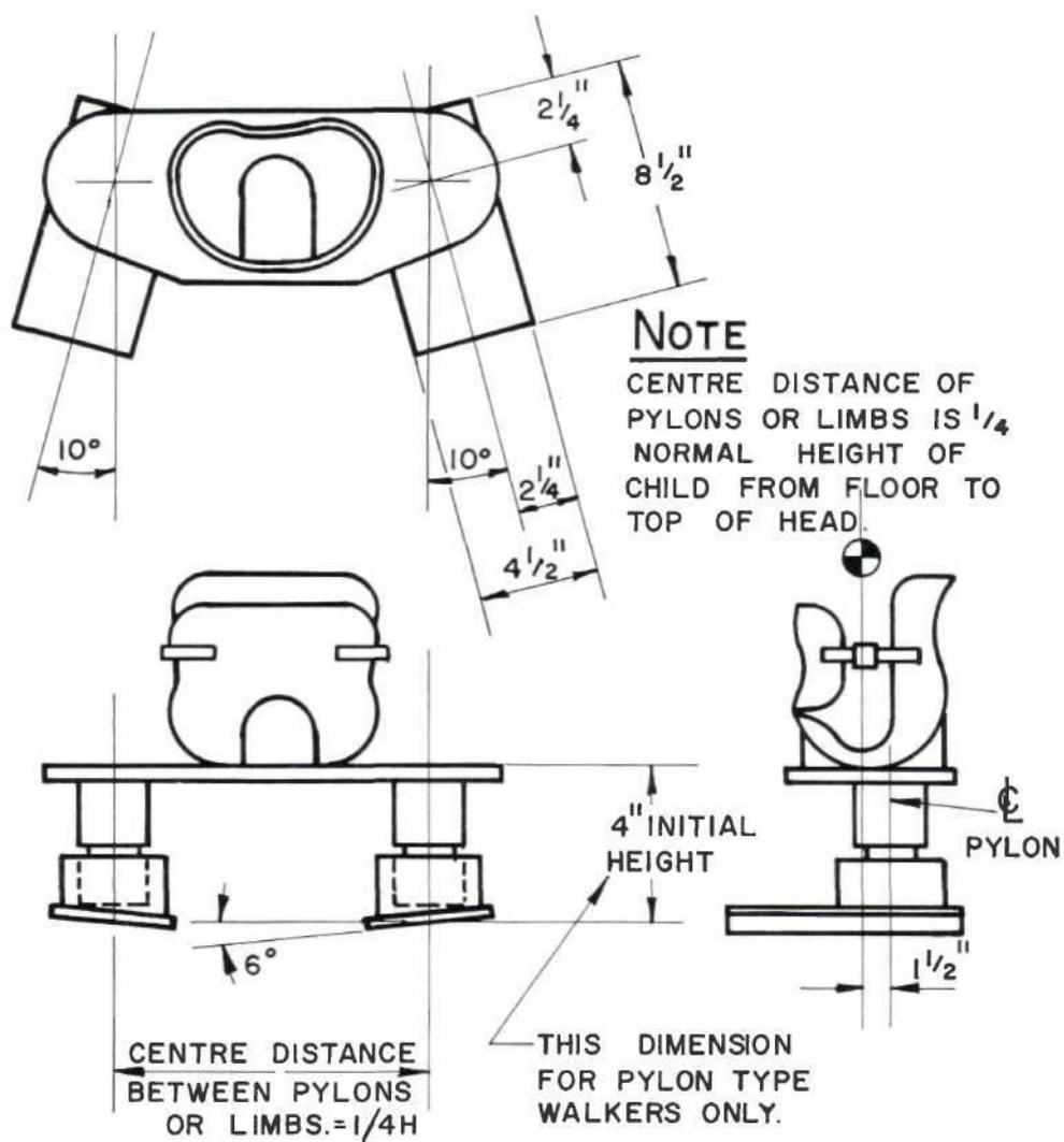
Fig. 2. Basic dimensions of the swivel walker.
