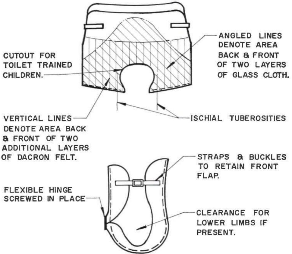
Fig. 5. Recommended socket configuration.
