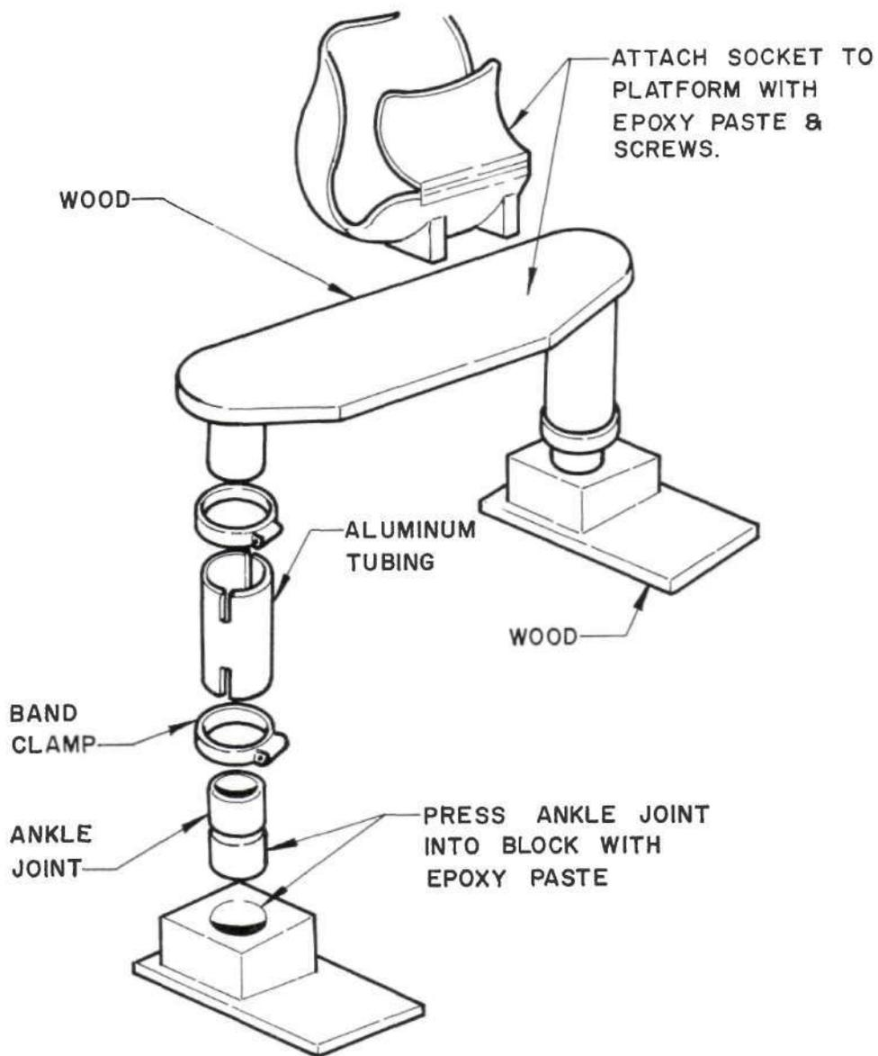
Fig. 6. Assembly of the swivel walker.
