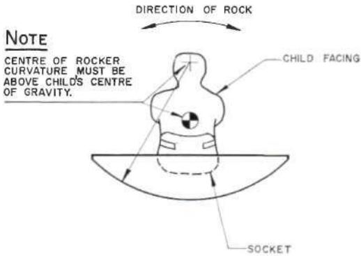
Fig. 9. Device for training patient to use the swivel walker. The lateral rocker enables the child to establish balance, to learn and practice the sideways rocking motion, and to establish a rhythm.
