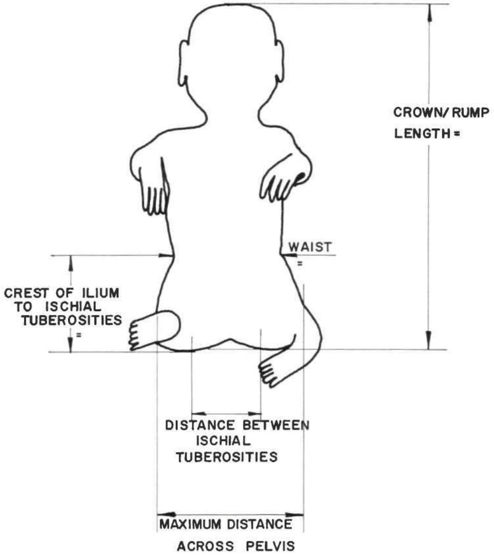
Fig. 3. Measurements required for fabrication of the swivel walker.
