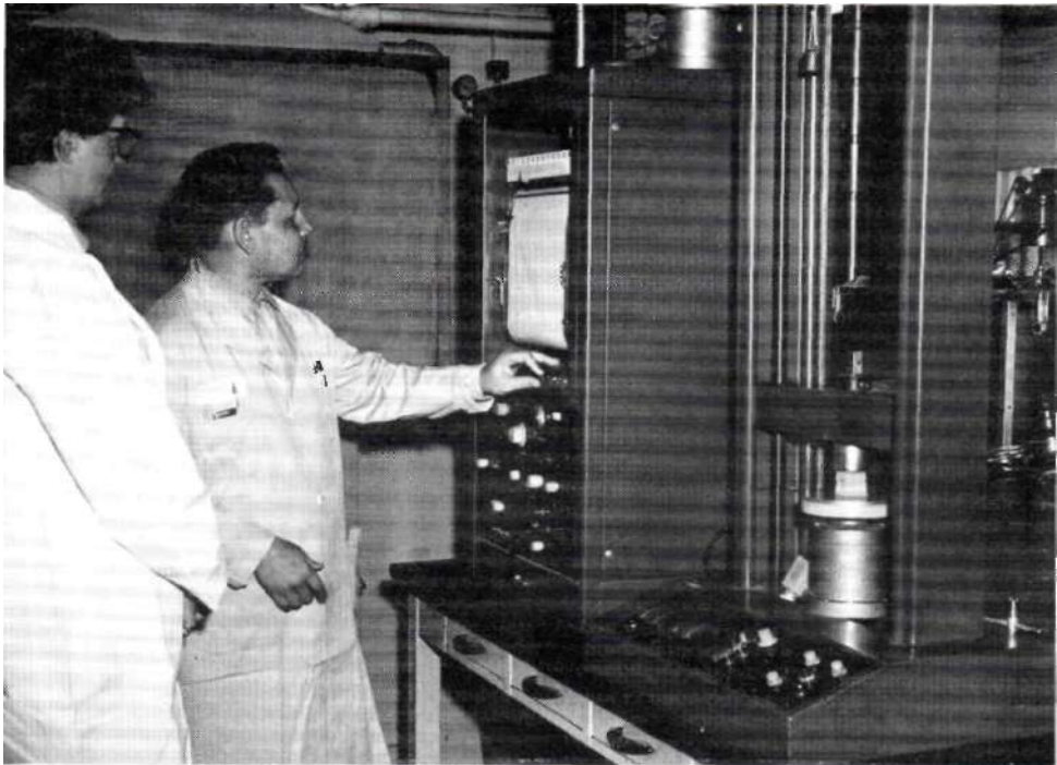
Fig. 1. Using a table model Instron Testing Machine to test a sample formulation. The forces can be read on the graph.
