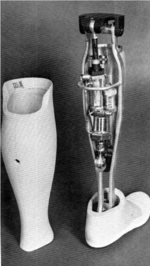
Fig. 20. "Hydra-Cadence" Artificial Leg with cosmetic cover removed.
