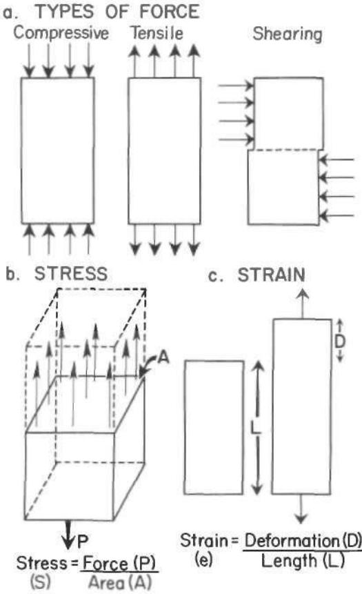
Fig. 1. Types of pure force—stress and strain.
