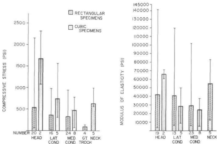
Fig. 5. Mean and range of variation in some mechanical properties of spongy bone from different regions of the femur. Compressive stress values in *pounds force per square inch*. *Gt. troch.* = greater trochanter; *Lat.* = lateral; *Med.* = medial; *Cond.* = condyle.
