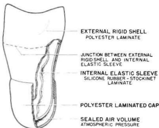
Fig. 6. Cutaway view of the air-cushion socket.
