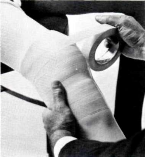
Fig. 9. Application of pressure using an elastic pressure-sensitive-tape wrap.
