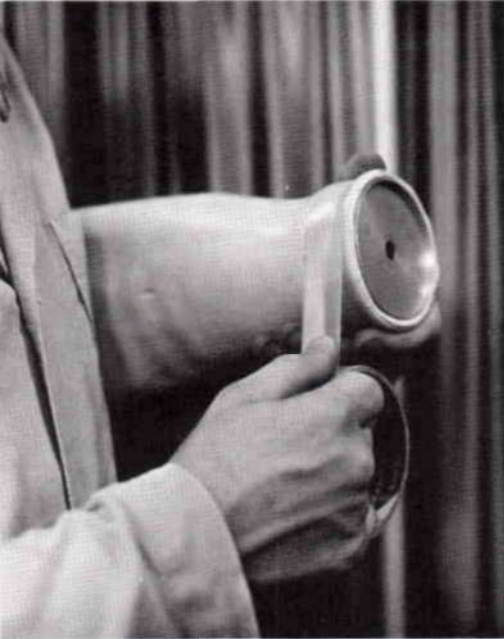
Fig. 12. Socket compressed against turntable with pressure-sensitive tape.
