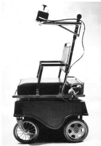
Fig. 7. Cart with solid rear wheels and new control unit.
