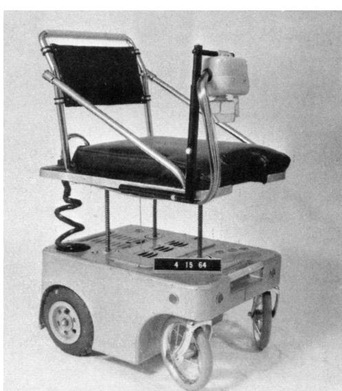
Fig. 2. Prototype II, CAPP electric cart.
