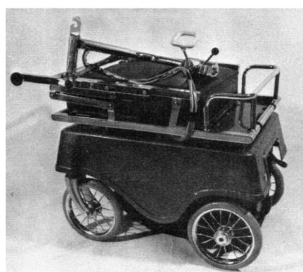
Fig. 5. Field-test cart folded.
