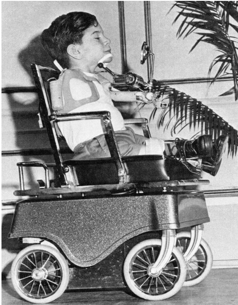
Fig. 1. The CAPP cart. Power is provided by a 12-v battery; direction is controlled by the chin-operated lever.
