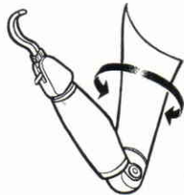
Fig. 7. Test for socket stability during arm rotation.
