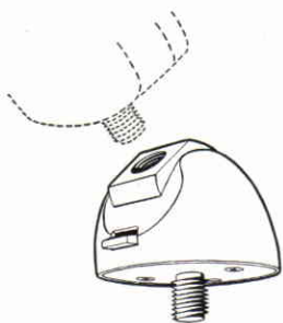
Fig. 8. Northrop-Sierra model B wrist-flexion device.
