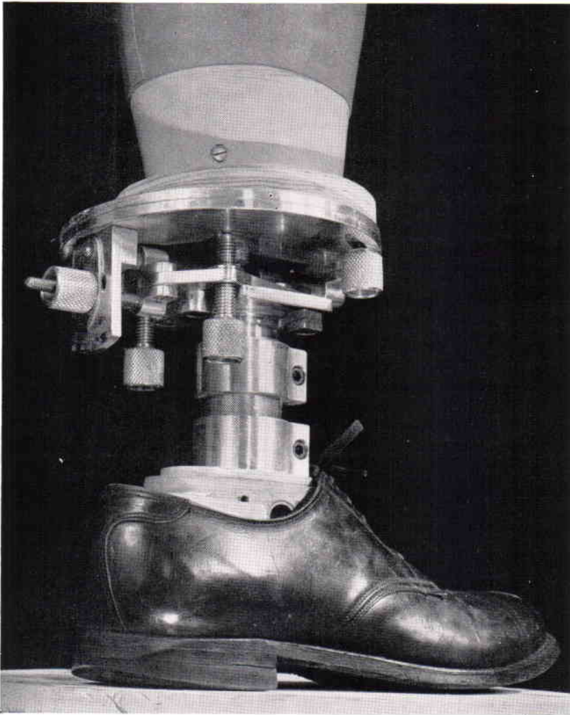
Fig. 15. Combination above-knee/below-knee adjustable leg in use as a trial below-knee prosthesis.
