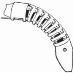
Fig. 9. One form of multi-segmented artificial finger. Complexity such as this leads to lateral instability.
