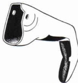
Fig. 10. Artificial finger of monocoque construction with fixed knuckle angles so chosen as to cause grasped objects to be drawn into the hand rather than rejected.
