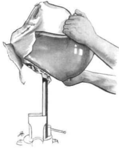
Fig. 22. Removing the socket from the mold.
