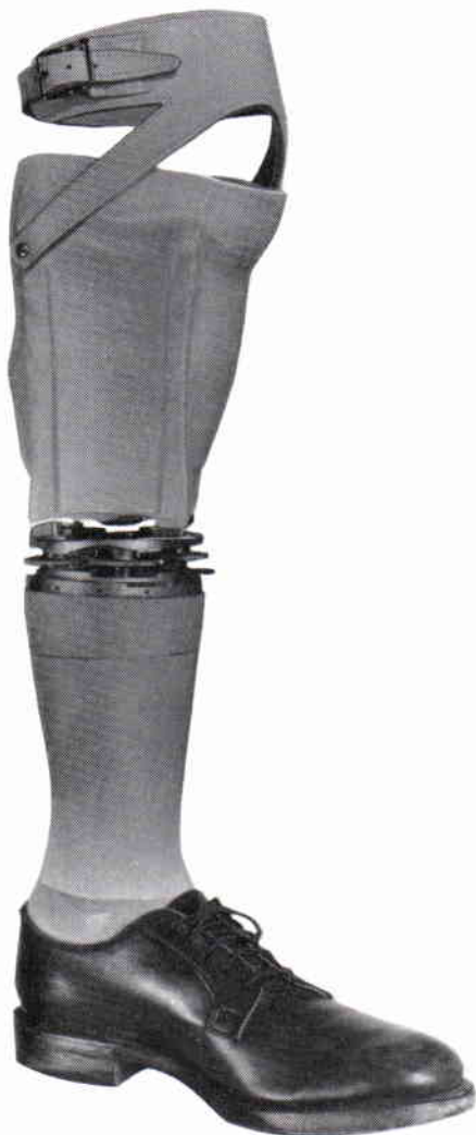
Fig. 17. The adjustable coupling used with a plaster-of-Paris below-knee temporary socket and unfinished shank. The three straps have the same cross-section as those used with the above-knee socket. The position of the carbon steel straps in both the above-knee and below-knee sockets should be reinforced with an extra plaster-of-Paris bandage wrap, as illustrated.
