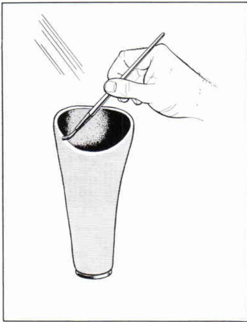
Fig. 7. Bonding the socket and forearm.
