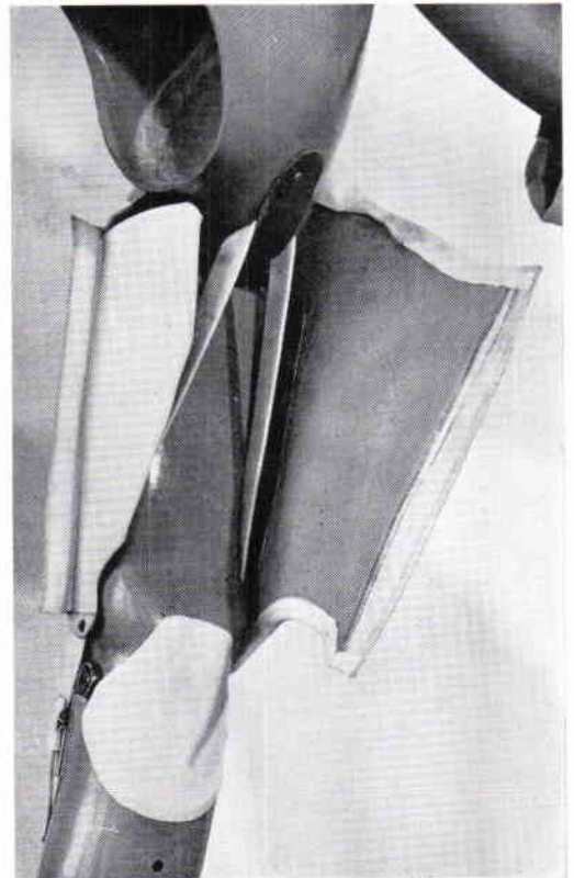
Fig. 32. Open view of completed thigh fairing.
