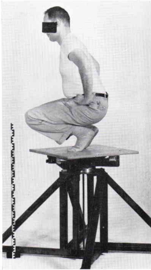
Fig. 20. Mass moment of inertia determination (squatting position).
