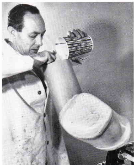
Fig. 17. Pouring polyurethane foam into cardboard form.
