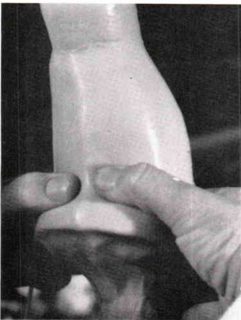
Fig. 42. Working resin into undercut areas.
