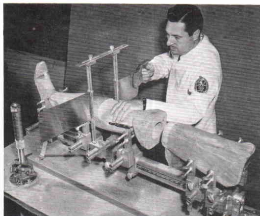
Fig. 9. The alignment duplication jig developed by the University of California Biomechanics Laboratory (San Francisco and Berkeley) to be used in conjunction with the adjustable leg shown in Figure 8.
