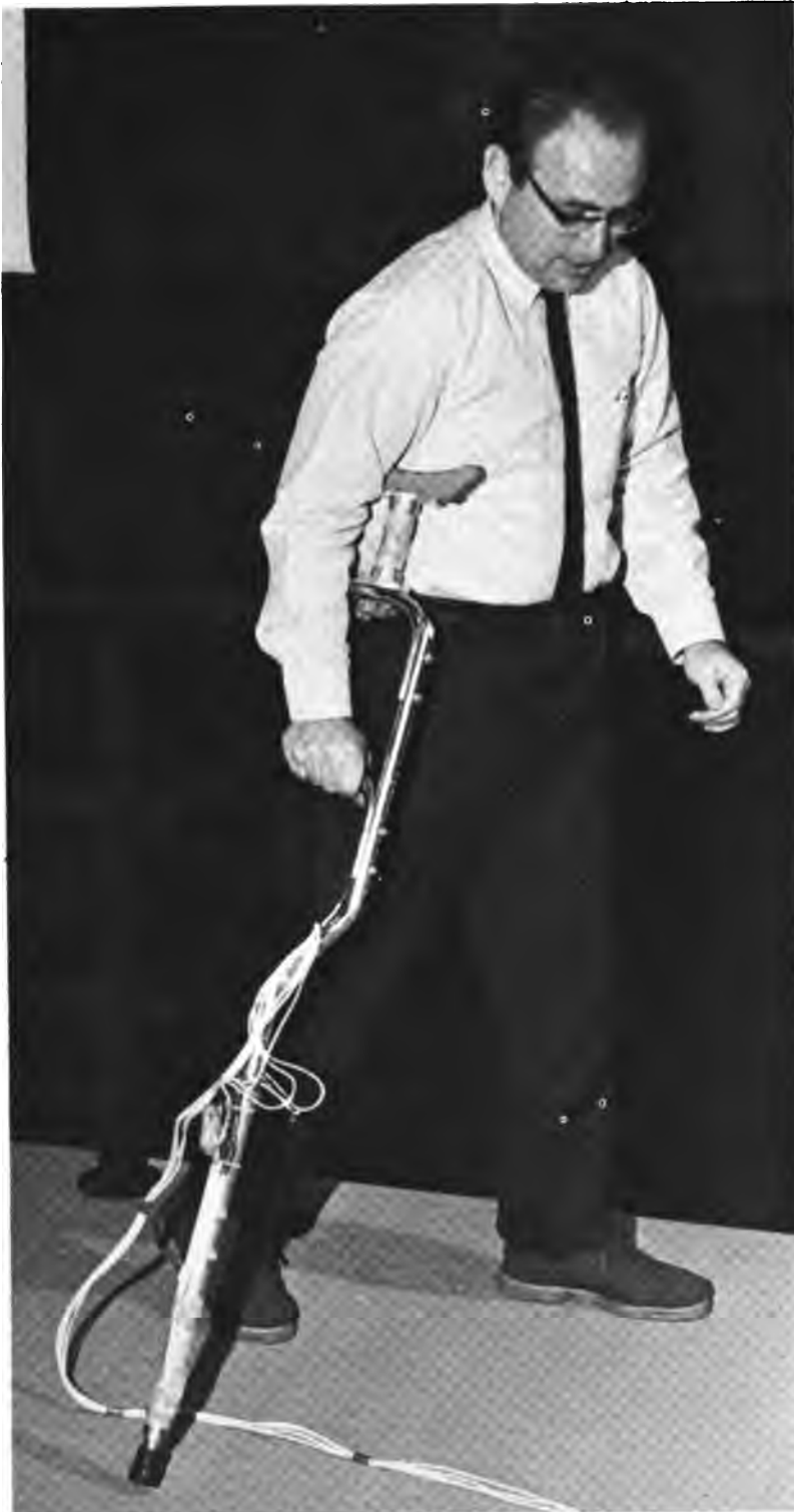
Fig. 12. Instrumented crutch developed at Case Western Reserve University.
