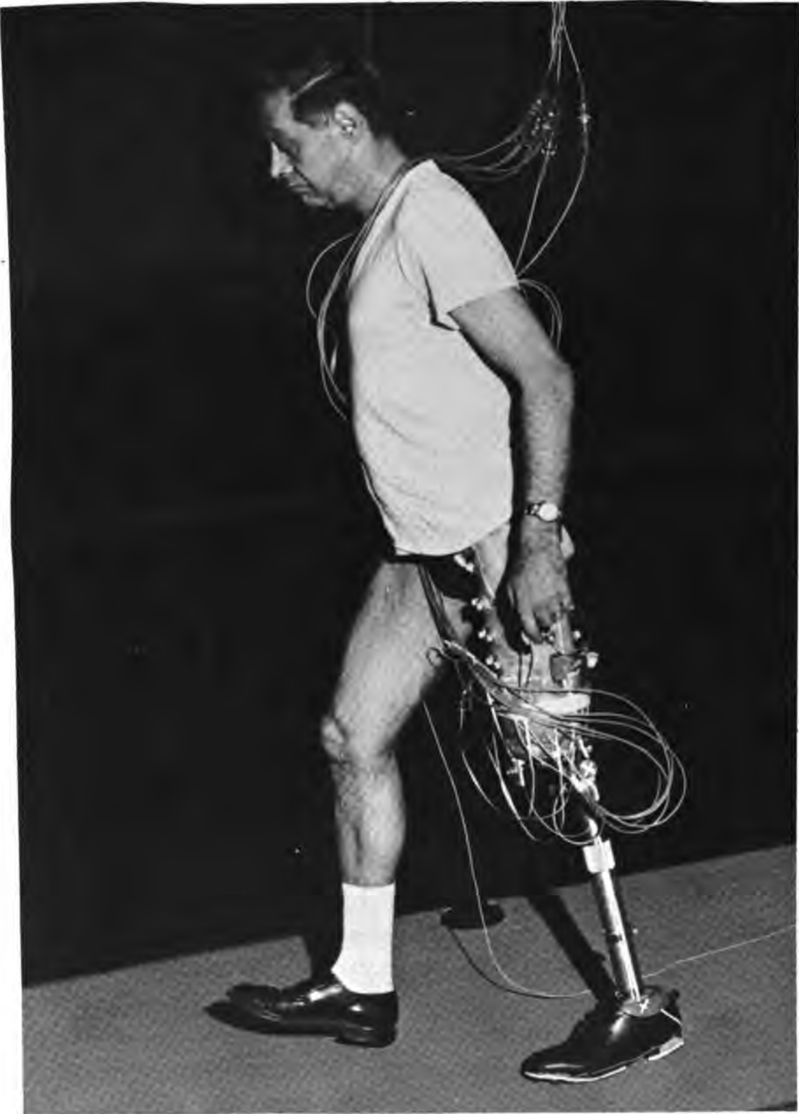
Fig. 5. Patient walking with NYU instrumented AK socket.
