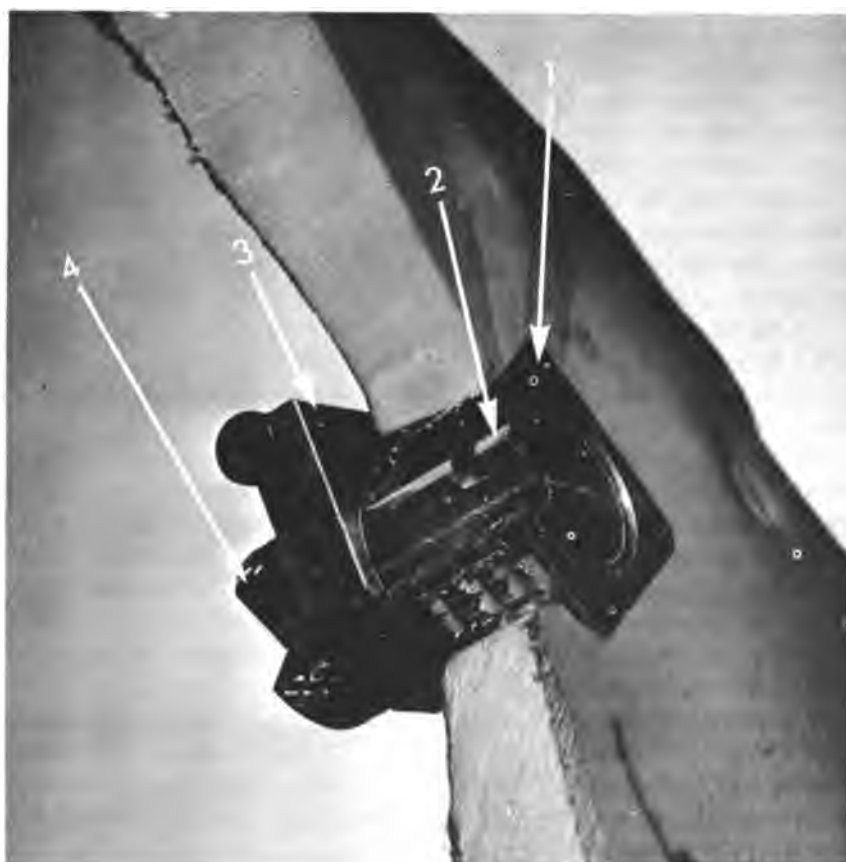
FIGURE 4.—Cutaway of socket and transducer mount.
