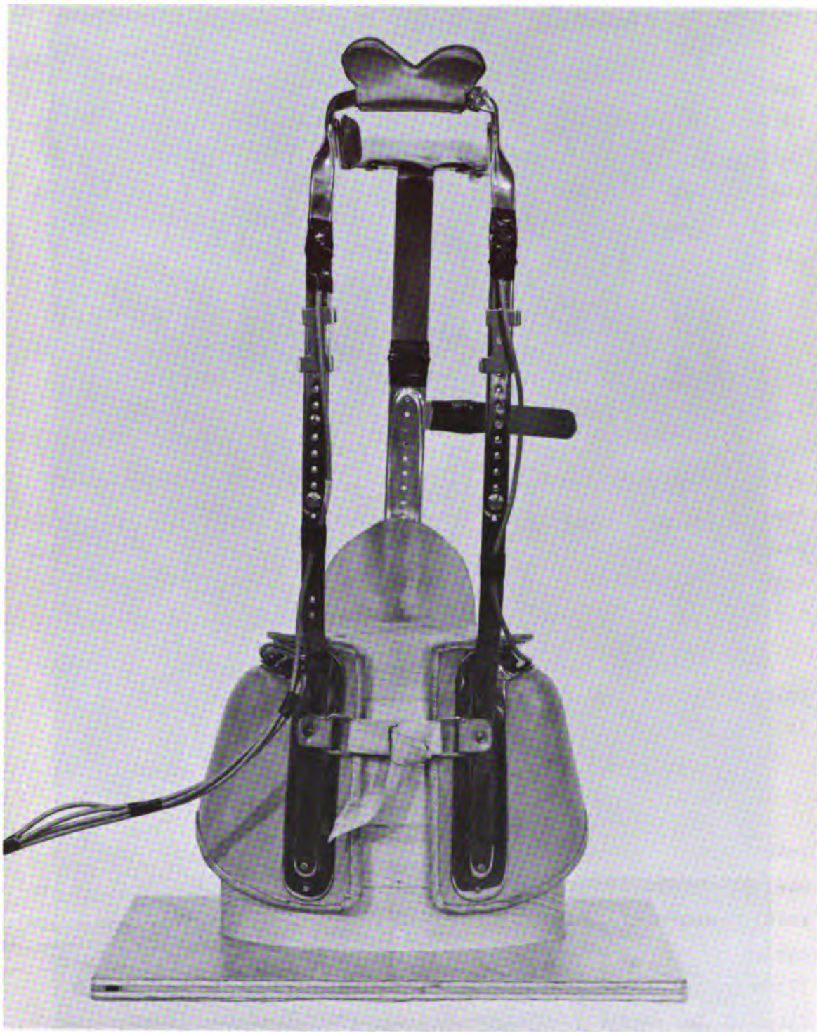
Fig. 10. Milwaukee Brace instrumented by University of Illinois.
