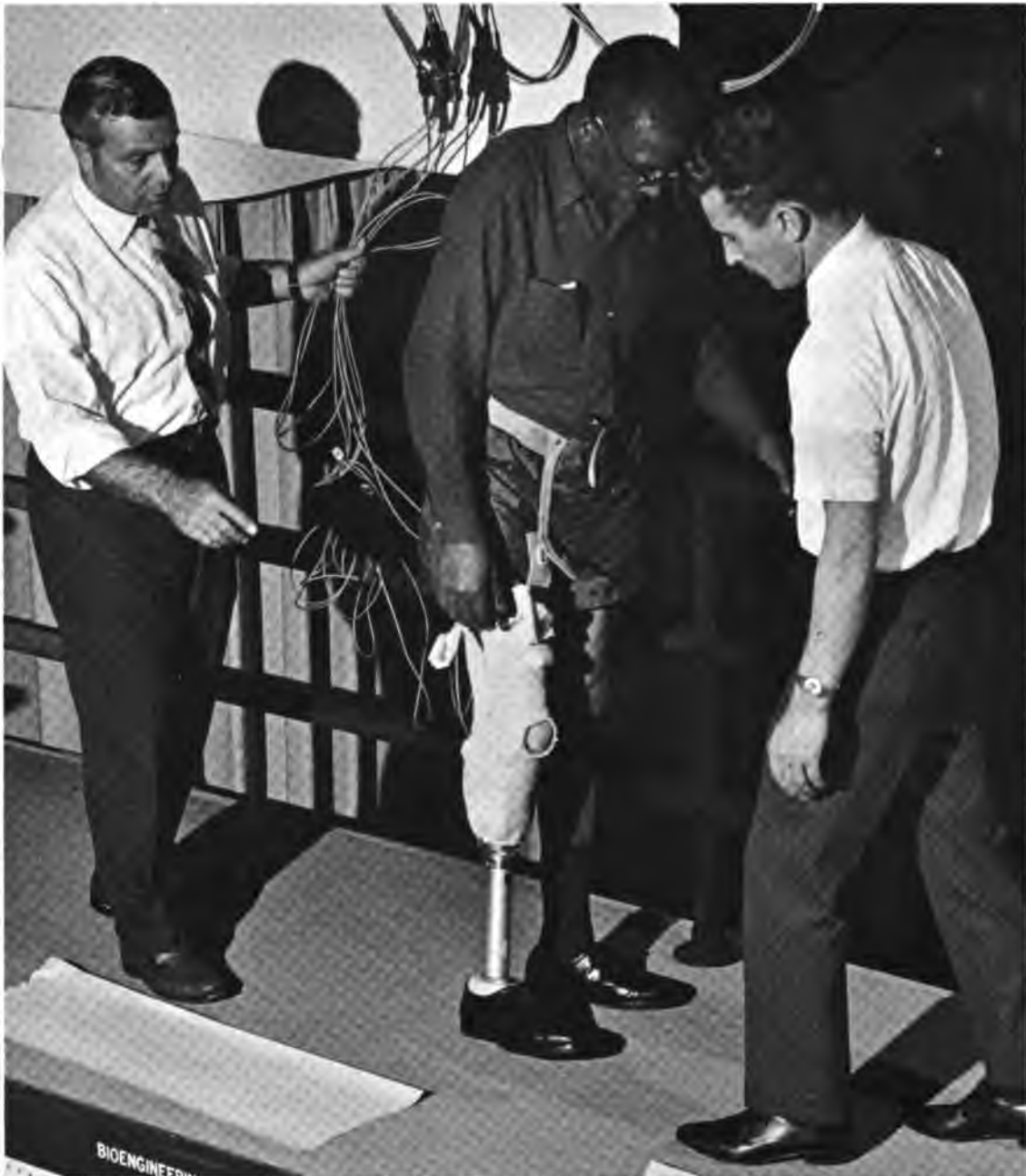
Fig. 6. Patient walking with VAPC-instrumented rigid dressing. Sensotec gauges are used here.
