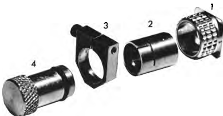
FIGURE 3.—Transducer mount parts.
