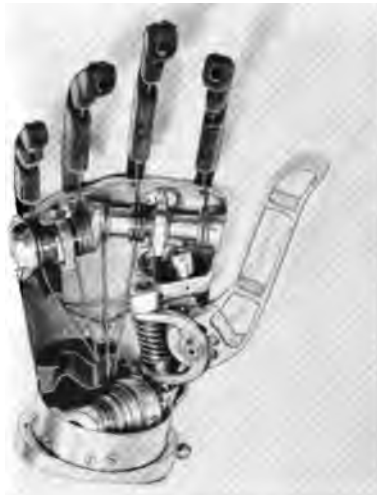
Fig. 17. Cable controlled, leaf spring mechanical hand.
