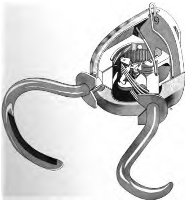
Fig. 21. Pull-to-close hook with force multiplier and locking mechanism.
