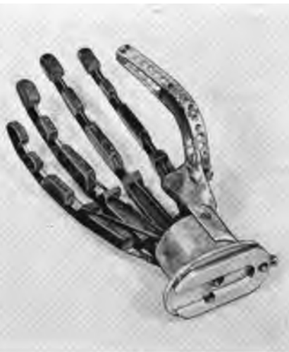
Fig. 18. Experimental flexible palm mechanical hand with quick wrist disconnect.
