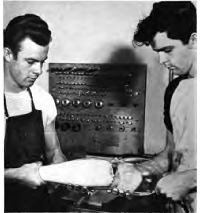
Fig. 28. Forearm section showing a polyvinyl alcohol bag being stretched over a completed lay-up.
