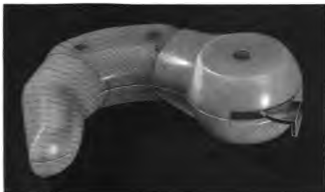
Fig. 77. Articulated nylon finger.
