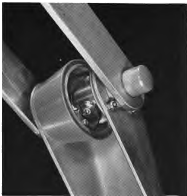
Fig. 12. Close-up of cone clutch type elbow lock.
