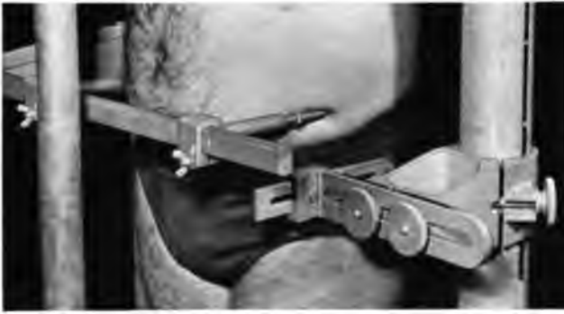
Fig. 31. Leveling attachment on fitting fixture.
