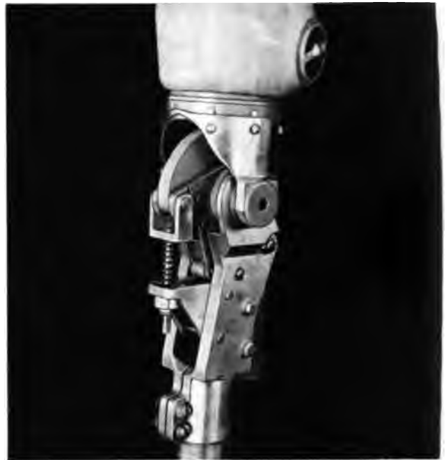
Fig. 24. Hydraulically actuated mechanical knee lock.
