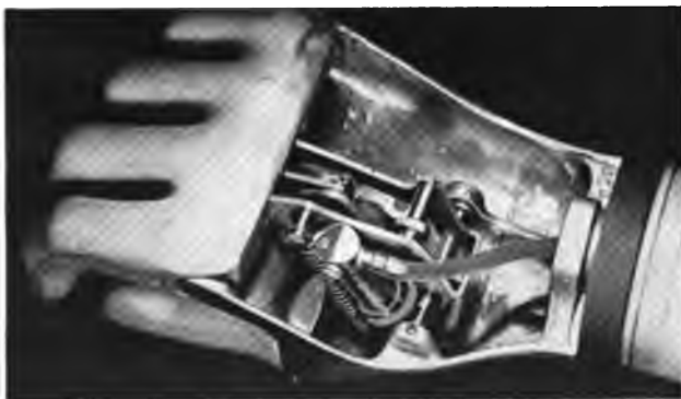
Fig. 75. Hand mechanism installed in a Miracle hand.
