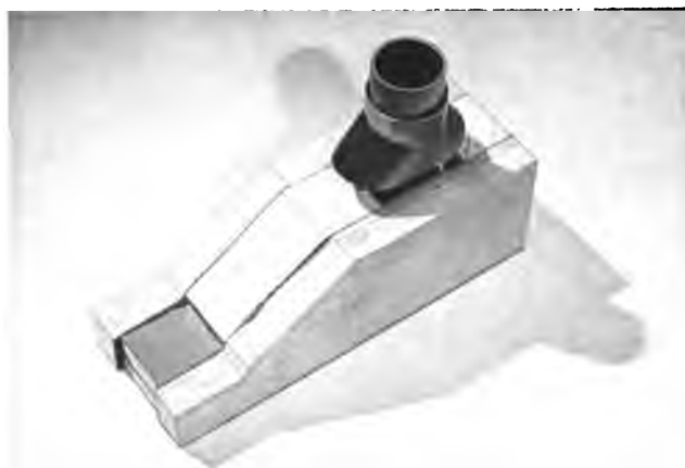
Fig. 83. Foot core assembly with side blocks and ankle assembly attached.
