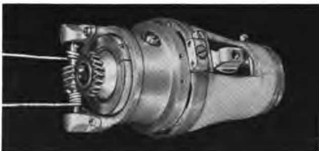
Fig. 125. Worm gear supination control for a Vard below-elbow cineplastic arm.
