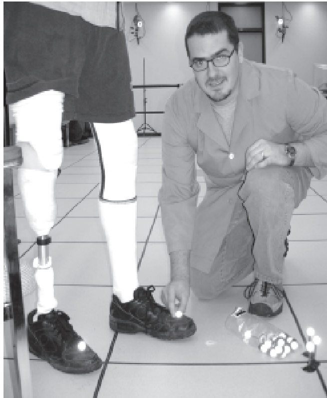
Andrew Hansen uses the VACMARL in the NUPRL area to examine the effect of roll-over shape on the alignment of transtibial prostheses.
