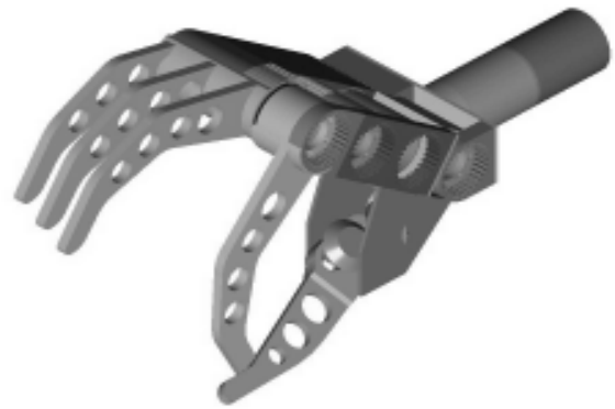
Fig. 1: 3D CAD drawing of our new multifunctional hand mechanism. Drawing shows how middle, ring and little fingers move together as a unit.
