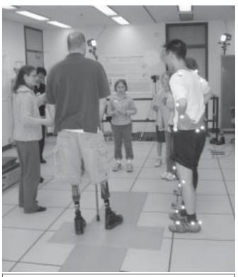
*Figure 3:* (From left to right) Stefania Fatone, Ph.D., Brian Ruhe, M.S., and Po-Fu Su, M.S., explain and demonstrate motion analysis using force plate and infrared cameras.
