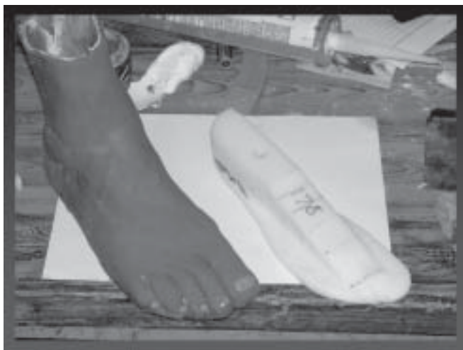
Cosmetic shell (left) fabricated from silicone and Shape&Roll Foot core (right). (Photograph courtesy of E. Pennington-Ridge)
