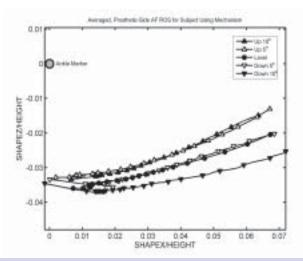
Figure 1: Averaged, single-limb-stance, ankle-foot roll-over shapes (ROS) for the prosthetic side of a single individual walking on our experimental foot and ankle mechanism on a level surface as well as on ramped surfaces with inclinations of +10, +5, -5, and -10 degrees. The x and y axes give coordinates of the shapes normalized by the user's height.
