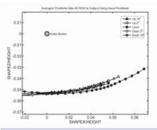
**Figure 2**: Averaged, single-limb-stance, ankle-foot roll-over shapes (ROS) for the prosthetic side of a single individual walking on his usual prosthesis on a level surface as well as on ramped surfaces with inclinations of +10, +5, -5, and -10 degrees. The x and y axes give coordinates of the shapes normalized by the user's height.
