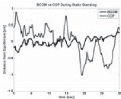
Figure 2: While an able-bodied subject stands as motionless as possible on a force platform, oscillations of the body center of mass (BCOM) and center of pressure (COP) about a relative equilibrium position—in this example, the mean positions of the BCOM and COP—can be observed. Both BCOM and COP show small displacements about the equilibrium point. (Data are courtesy of the VA Chicago Motion Analysis Research Laboratory.)
