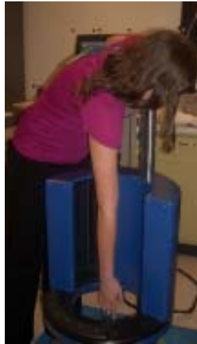
A CLSHS science student positions her arm in the B-K Scanner, which converts 3-dimensional laser measurements of exterior objects to digital files for fabrication.
