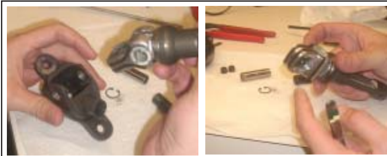
Disassembling the Mauch Hydraulic Ankle: The left photo shows the Housing (left) with the Piston Rod within the Shank Tube (right) removed. Visible in the base of the concave-shaped Housing is the gravity-activated Ball that closes the Control Port and prevents the flow of hydraulic fluid when the Shank is at vertical during mid-stance. The right photo shows the layered Chamber Sealings at the base of the Piston Rod. Fluid from the Back Chamber opens the Flap Valve at the site of the bore in the center.
