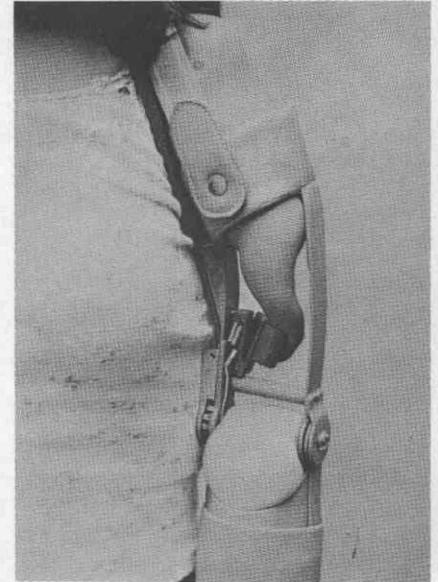
Fig. 6. Microswitch which is operated by the movements of the one finger phocomelia.
