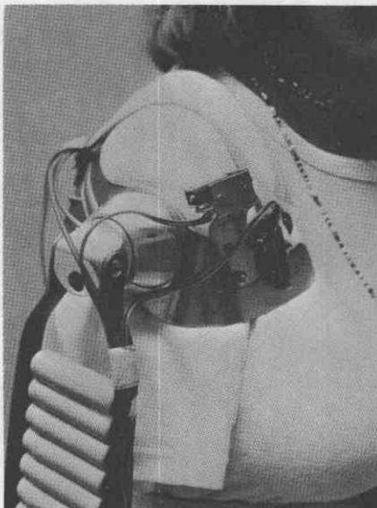
Fig. 7. Hybrid prosthesis in bilateral amelia with pneumatically lockable shoulder joint (controlled by valves in the left side) and pressure and traction microswitches for gripping and forearm rotation. Built-in accumulators fitted to the frame of the right upper arm.
