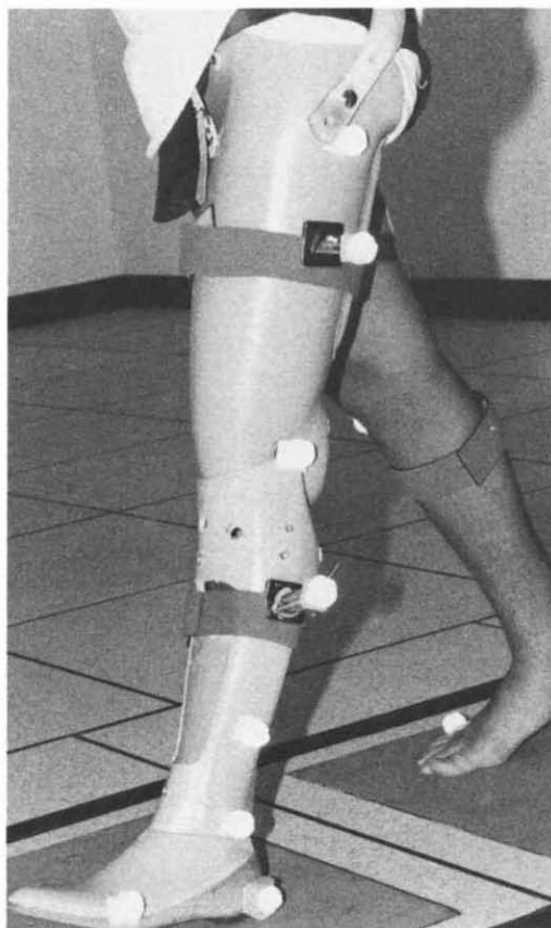
Figure 1. Completed experimental prosthesis; shown during testing in the Kinesiology laboratory.
