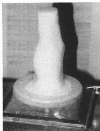
Figure 6. The outer socket frame is vacuum-formed over the inner socket.
