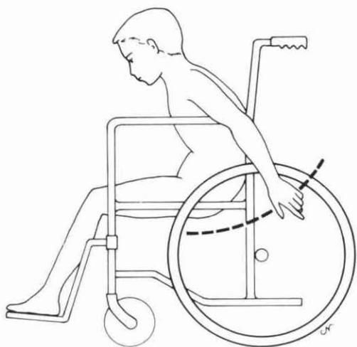
Figure 32. The “hammock” style upholstery on standard wheelchairs encourages a “slouched” sitting posture. That posture is almost necessary for a good hand-on-wheel power stroke.
