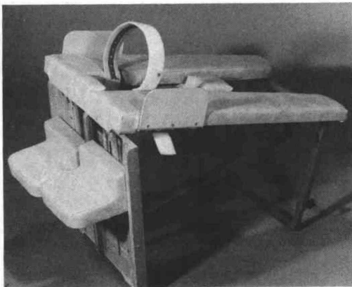
Figure 37. This is the positioning fixture which helps us obtain an impression with the alignment characteristics we hope to achieve in the finished S.S.O. The hip flexion angle can be varied. The knee supports are moved to the proper position for each child's impression. The waist belt helps to reduce lumbar kyphosis.
