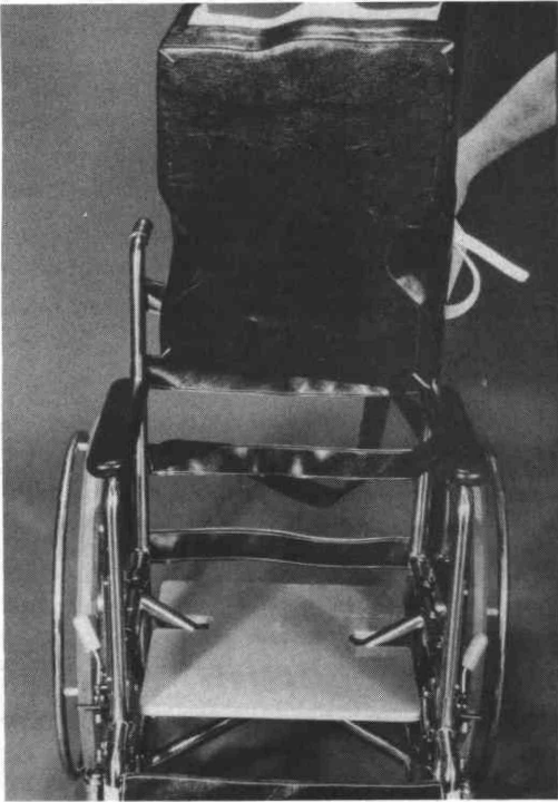
Figure 35. This photo shows an example of how to shape the base of a seat and use straps instead of standard upholstery to recess the seat into the wheelchair for better access to the wheels.
