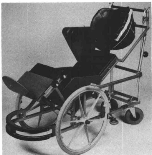
Figure 30. This cradle type headrest is mounted so that it can be pivoted by means of a small wheel-crank. The child turns the wheel-crank to change weight bearing areas and to change the direction of her gaze.
