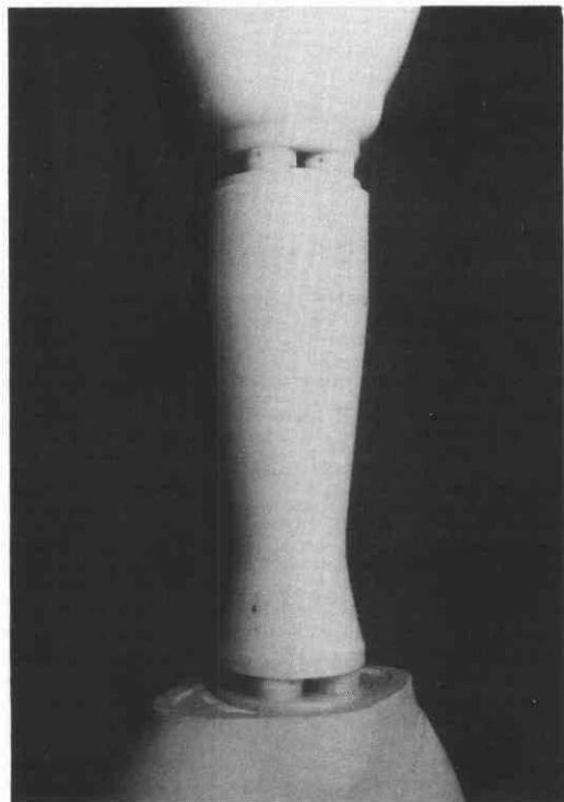
Figure 5A. A rotational molded tapered column made from nylon.
