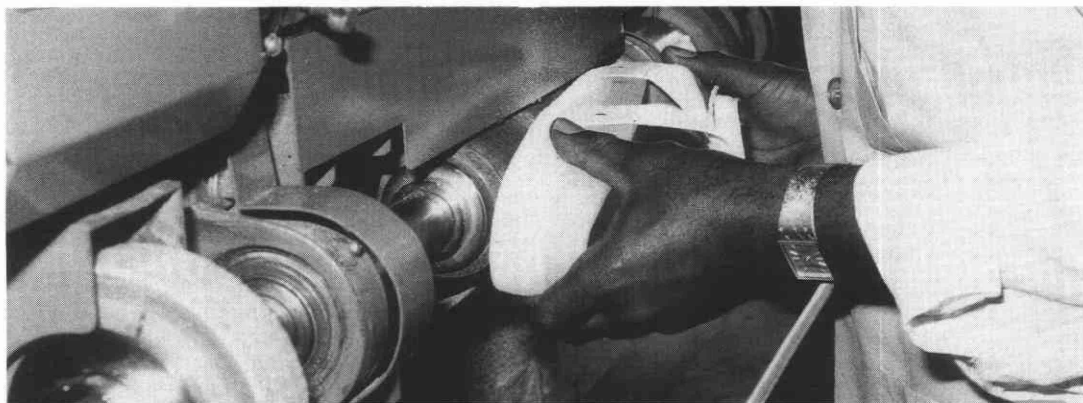
Figure 6. The bottom of the sandal is ground flat under heel, arch, and metatarsal heads after the heel wedge is glued on. The area under the toe is ground up to form the rocker.
