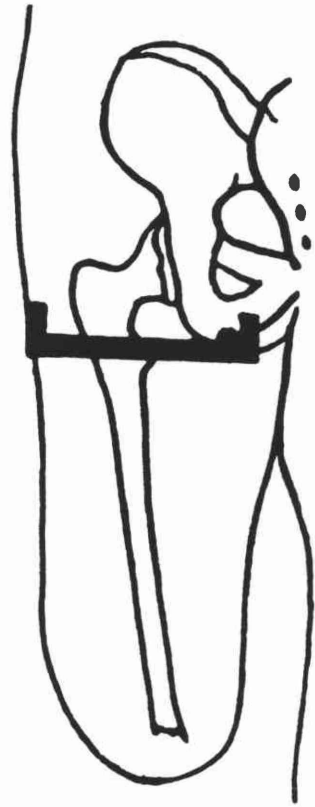
Figure 13. Ischial Tuberosity ML (IT), medial-lateral diameter measurement for Narrow ML Socket. 5
