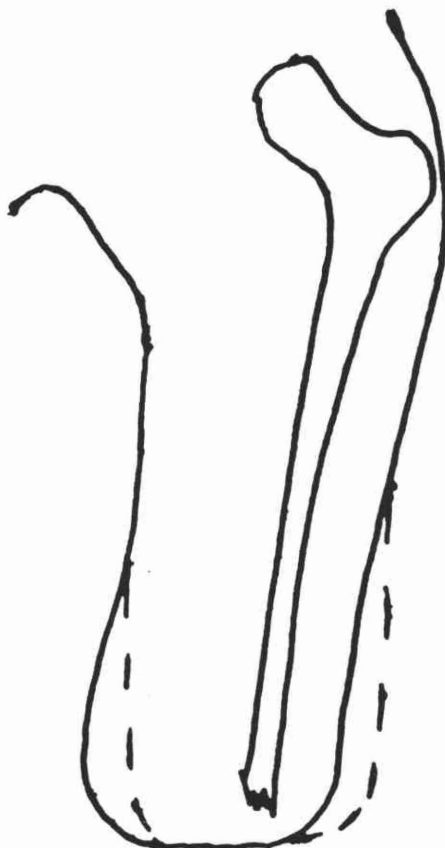
Figure 10. Centralization of the femur, as proposed by Dan Shamp for Narrow ML Socket. 5
