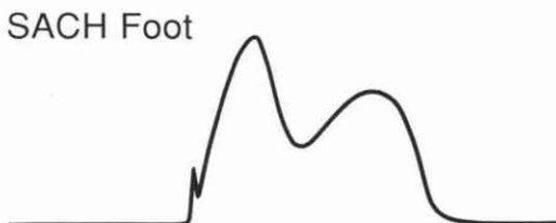
Figure 14. Stance forces generated in the same individual on his prosthetic side using a S.A.C.H. foot.
