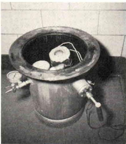
Fig. 5. Furnace, mold, and container for pouring aluminum in vacuum.
