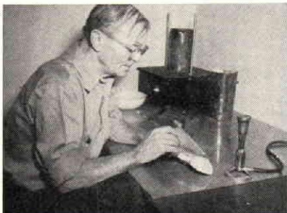
Fig. 3. Attaching web to wax pattern for footplate.
