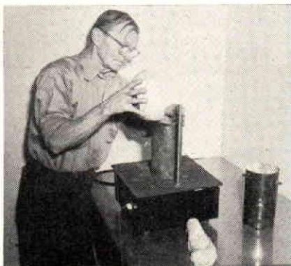
Fig. 4. Investing wax pattern in plaster paris-sand mixture.
